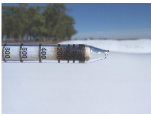
Figure 3. Detail of colorimetric tube showing a concentration of 200 ppm phosphine.
